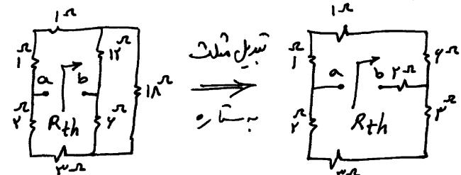
$$R_i = \frac{R_b R_c}{R_a + R_b + R_c} = \frac{4 \times 12}{4 + 12 + 1A} = \frac{48}{17} = 2.8^{\Omega}$$
